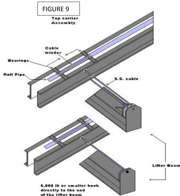
7. Thread the taped end of cable up between carrier beams and cable winder. Push taped end of cable through hole in the cable winder until cable comes out of pipe.
