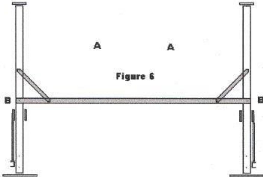
5. Carry the leg assembly to final location of install. This will allow the unit to be placed for leg adjustment and to check to assure that its level.
